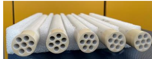
L= 250 mm OD: 25 mm, ID: 6 mm, 7 Channels,
