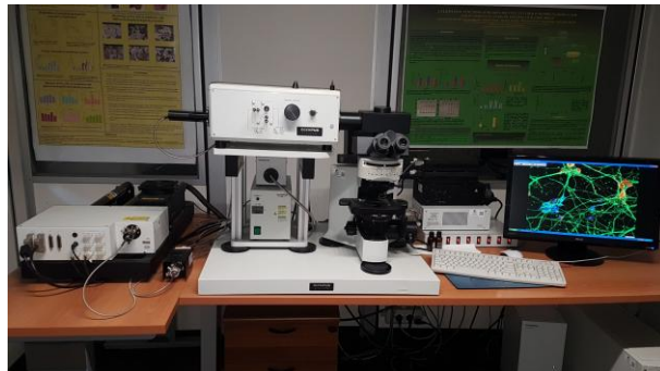
Laser Scanning Confocal Microscopy for the characterization of membranes and cells in bioartificial system.
