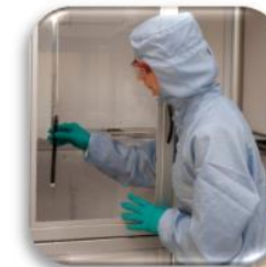
4. Dip-coating of electrode with semi-automatic dip-coater and firing
