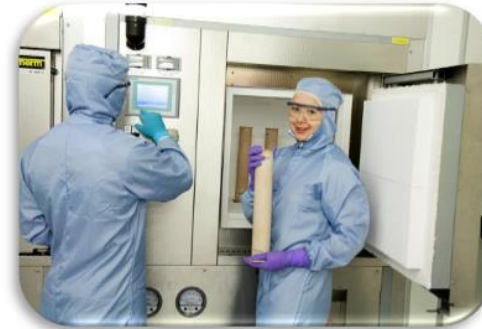
3. Co-sintering of electrode/electrolyte
